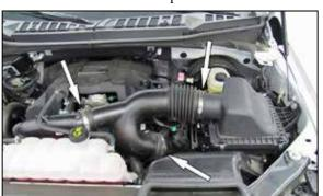
3. Loosen the three hose clamps that secure the factory intake tube and then remove the intake tube from the vehicle.
