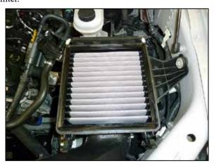
5. Install the provided AIRAID® air filter into the lower air filter housing.
