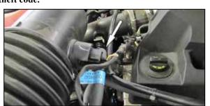
2. Disconnect the inlet air temperature sensor.
