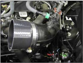
6. Install the provided coupler hose onto the turbo inlet tubes and secure with the provided hose clamps.
