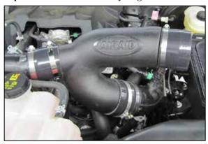
9. Install the AIRAID® intake tube assembly into the coupler and adjust for best fit, then secure the tube with the provided hose clamps.
